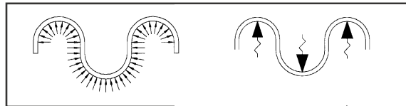
Hydroformed Mechanically Formed Corrugations are fashioned into the tube either mechanically or hydraulically, called "hydroforming." Hydroforming corrugations evenly distributes stresses; mechanically forming corrugations creates concentrated stresses
